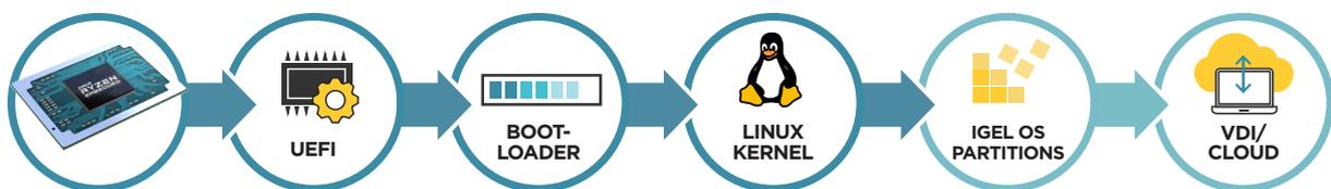
IGEL’s chain of trust verifies each step of the boot-up process from the IGEL-branded hardware/UEFI to the destination VDI host or cloud workspace delivered by Citrix, VMware and more. A secure browser can be configured for safe user access to web apps and cloud-based DaaS offers including Amazon Web Services (AWS) and Windows Virtual Desktop (WVD) from the Microsoft Azure cloud.
