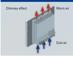
Our innovative application of the chimney effect makes it possible to run up to  $+65\,^{\circ}\text{C}$ . The integrated heater allows the start of the devices from -40  $^{\circ}\text{C}$ .
