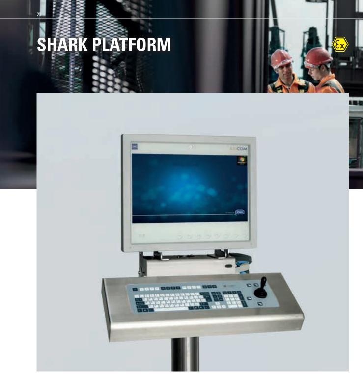
SHARK operator station with barcode scanner and integrated RFID module
